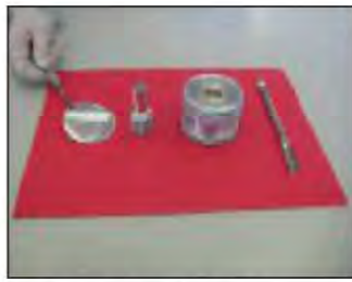
The tin disk is rested on the filter paper.
