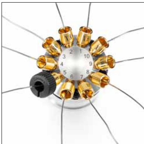
Figure 8. A 10-port valve completely connected with Viper capillaries. Note that the black knurl can be removed easily after plumbing.
