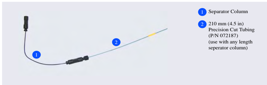
Figure 4 Tubing Connections for Separator Column Only
