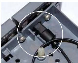
Figure 5 Column Outlet Fitting Installed in Column Cartridge
