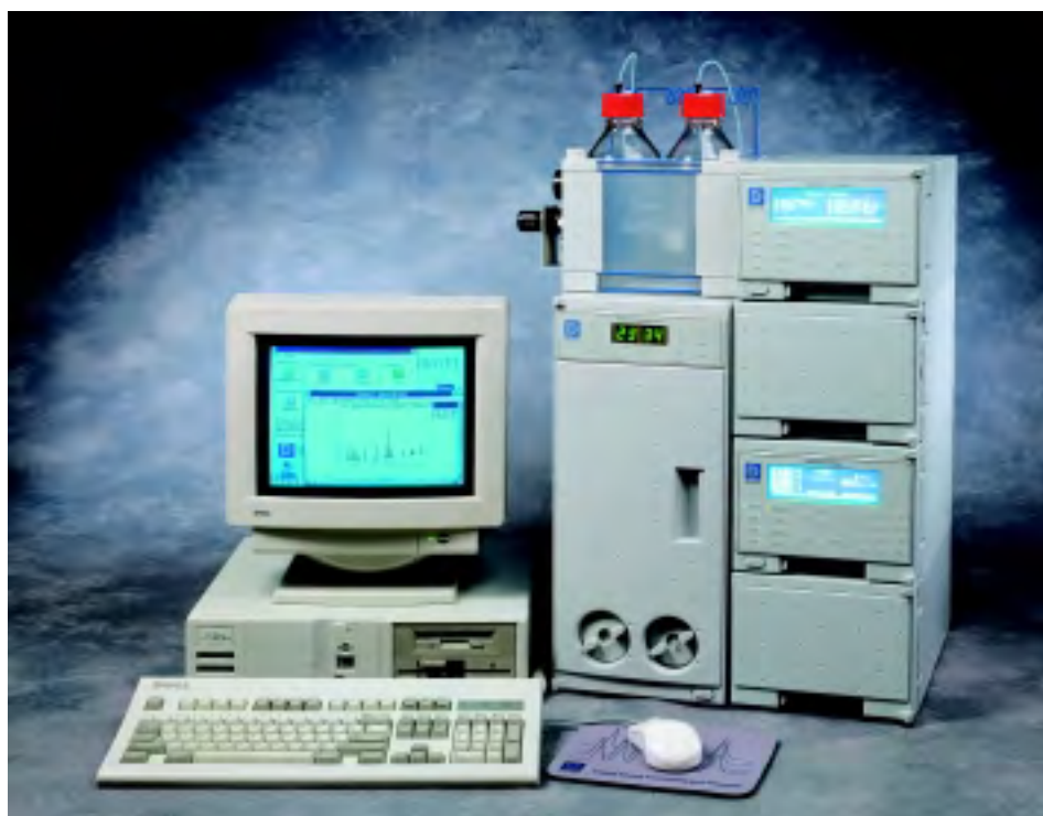
Figure 11 The Dionex PEEK-based DX-500 BioLC is designed to analyze DNA samples using Dionex protocols.
