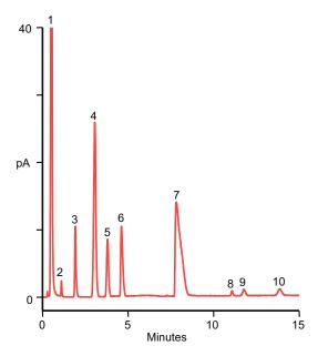
Figure 1: Separation of common anions and cations under standard salt-gradient conditions. Peaks 1: phosphate, 2: sodium, 3: potassium, 4: chloride, 5: malate, 6: bromide, 7: nitrate, 8: citrate, 9: fumarate, 10: sulfate, 11: magnesium, 12: calcium.
