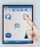
The Master SHS can be fully controlled directly by the touch screen display or the driver of the CLARITY Chromatography Station or by using the standalone software, SHS Manager.
